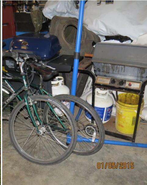
improper storage of propane tanks
